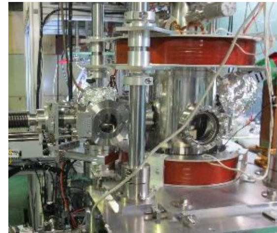
Load-lock chamber multi-sample holder (5 pic.)
