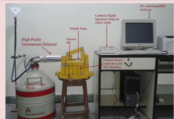
Experimental Setup of PAS in the Laboratory.
