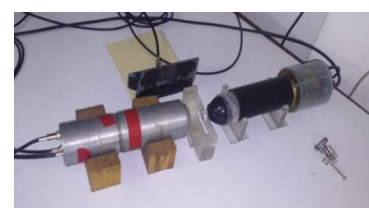
Figure 2: PALS experimental device. FWHM of 202 ps.
