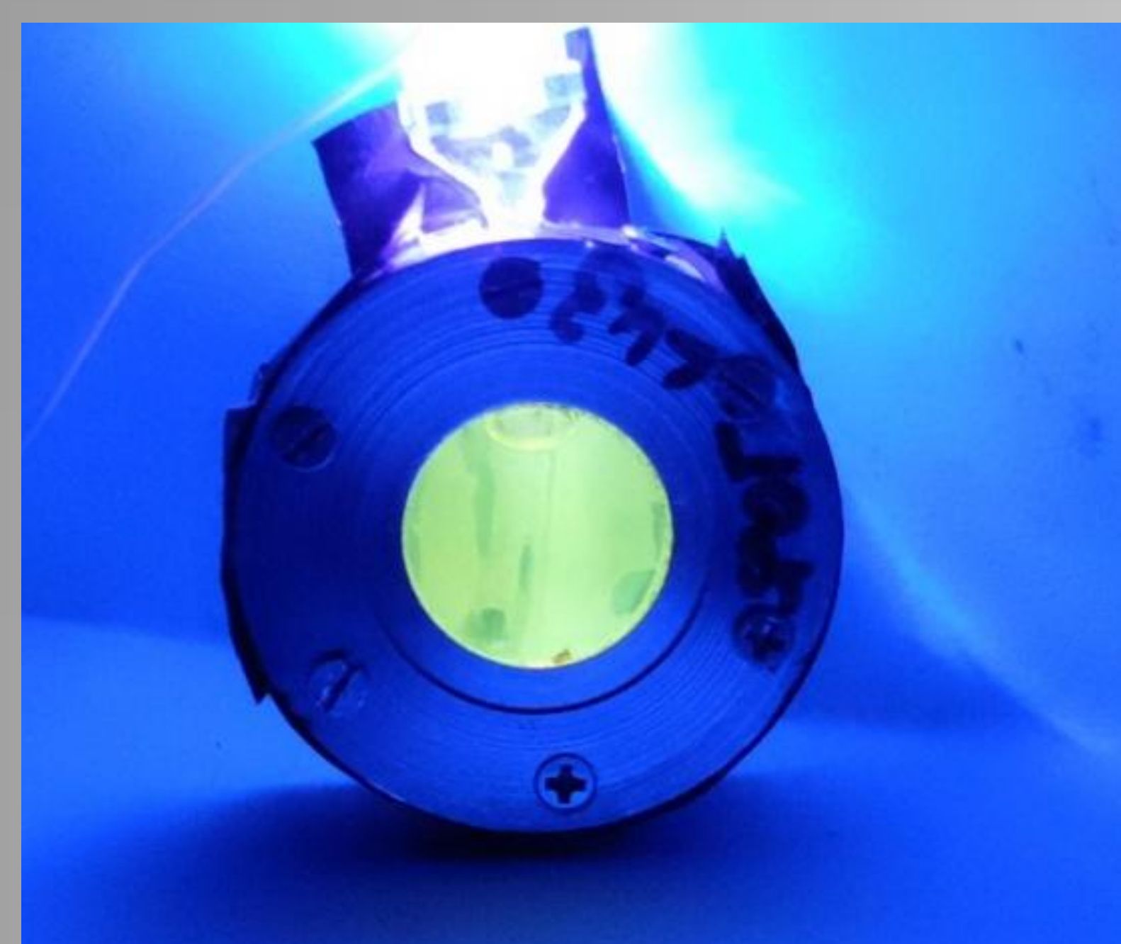
Fig. 1 The configuration of the aluminium chamber with the light source (LED, 405 nm, 0,27 mW cm -2 , in the middle of chamber)
