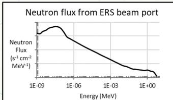
Upon entering the ERS, the neutron and photon beams have an extent of about 20 x 30 cm<sup>2</sup>. The neutron beam fast-to-thermal ratio is ~15.<sup>[2]</sup>
